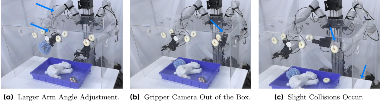
Figure 8 Causes of Longer Grasping Duration for Kinova Dual-Arm Robot in the Confined Space Grasping Experiment.
